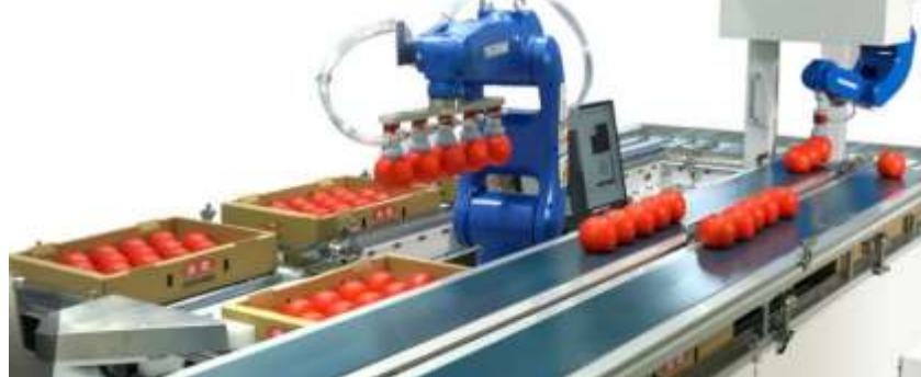
Handling of tomatoes with small robots MotoMINI
